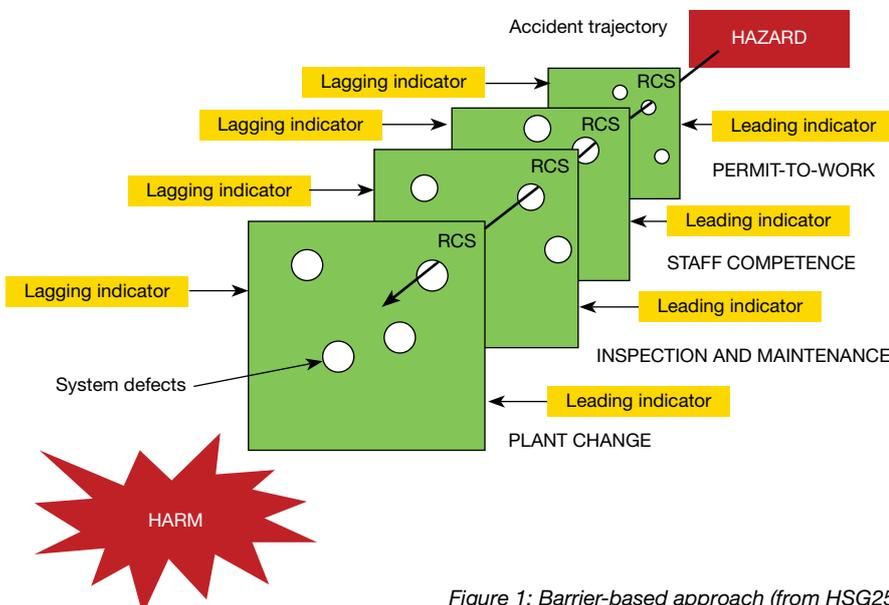
Figure 1: Barrier-based approach (from HSG254)
