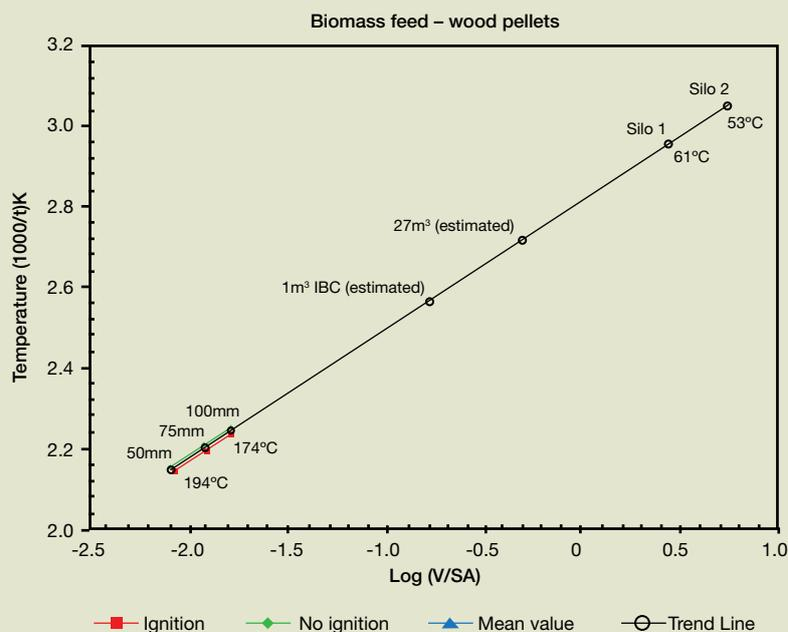
Figure 1: the critical ignition temperatures for a wood pellet extrapolated from small-scale basket testing to large-scale bulk storage silo conditions.
